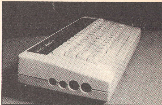
The four sockets at the right hand edge of the case provide UHF and composite video outputs as well as the RGB and cassette I/O connectors.
